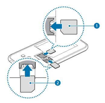
► Single SIM models: Insert the SIM or USIM card with the gold-coloured contacts facing downwards.
