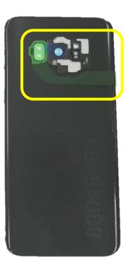
Before re-assembling, the outside tape & inside tape & finger print sensor tape should be changed.
