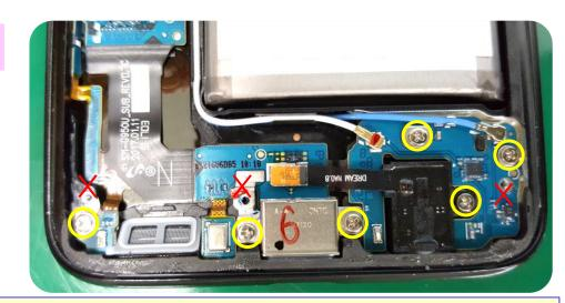
\* Do not confuse the screw holes for rear cases on the SUB-PBA.
