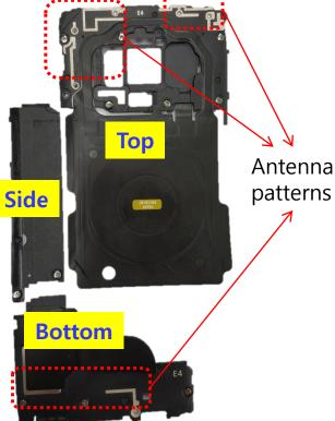
**Note:** Watch out not to give any damage on the antenna patterns in rear case.
