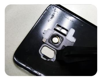
Do not push the finger print sensor from the backside to detach the finger print sensor.
