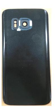
Before re-assembling, the outside tape & inside tape should be changed.
