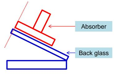
Close to the bottom of back glass (Do not go out of the back glass)
