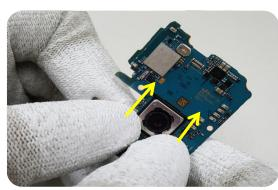
1) Remove Front cam / IRIS cam module & sensor FPCB & motor using top-rounded tweezer.
