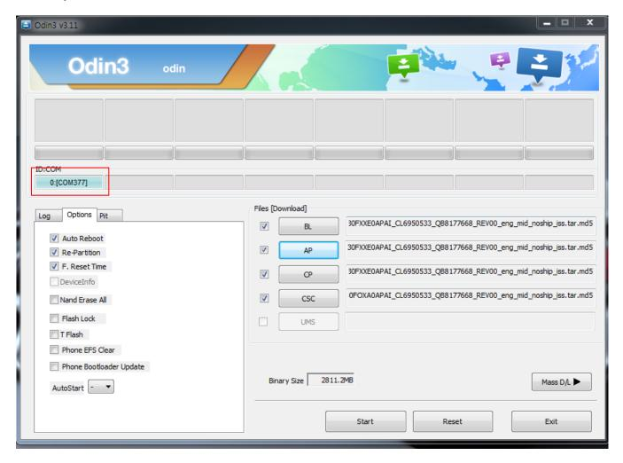
**4**. Start downloading the binary files into the device by clicking Start button on the screen. The green colored "PASS!" sign will appear on the upper-left box if the binary files have been successfully downloaded into the device.
