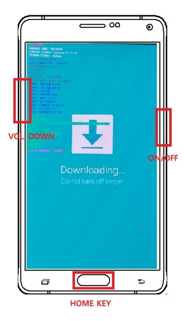
3. Connect the device to PC via Data Cable. Make sure that the one of communication ports [ID:COM] box is highlighted in sky blue. The device is now connected with the PC and ready to download the binary files in it.
