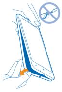
2. Make sure the contact area is facing down, and push the memory card into the memory card slot until it locks into place.
