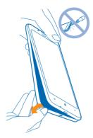
2. Make sure the contact area of the SIM is facing down, and push the SIM into the SIM slot.
