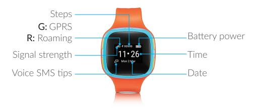
When the watch is roaming, the right side of the signal bar will appear "R". At the same time, prompt information will display in the massage bar in the application. **Note:** Consult the local operators to open the roaming service.
