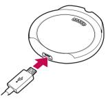
3 Place the watch on the charging cradle and make sure that the charging terminals are aligned with each other.
