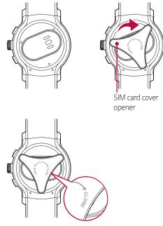
Foreign materials on the SIM card cover sealing pad or SIM card cover may allow water to get into your watch. Keep the cover clean and remove any foreign material before replacing the cover.
