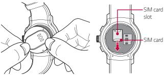
3 With the gold contacts facing down and the SIM card positioned as shown below, slide the Nano SIM card in to the SIM card slot.
